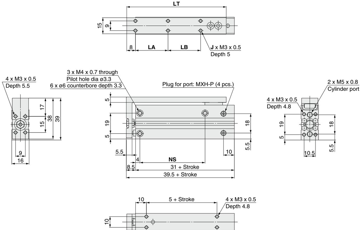
Note 1) Refer to "Specific Product Precautions" for mounting of the Compact Slide and a workpiece.
