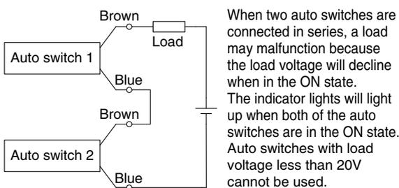
When two auto switches are connected in series, a load may malfunction because the load voltage will decline when in the ON state. The indicator lights will light up when both of the auto switches are in the ON state. Auto switches with load voltage less than 20V cannot be used.
