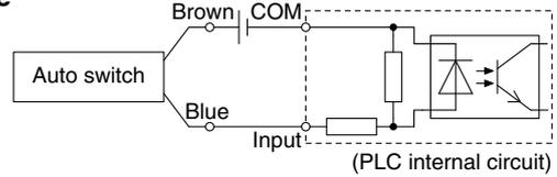
Connect according to the applicable PLC input specifications, as the connection method will vary depending on the PLC input specifications.
