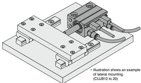
\* Illustration shows an example of lateral mounting. (CUJB12 to  $\varnothing 20$ )
