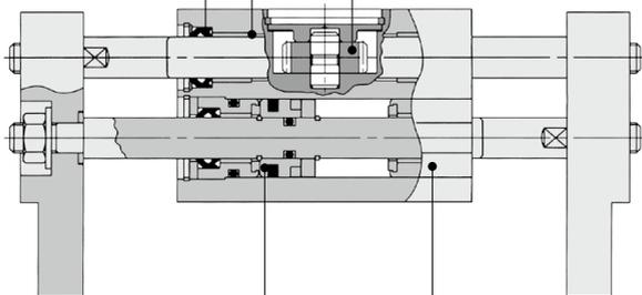
A large amount of gripping force is provided through the use of a double piston mechanism, while maintaining a compact design.
