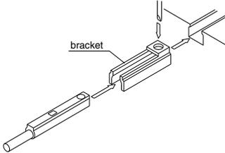
Note) Use a watchmaker's screwdriver with a grip diameter of 5 to 6 mm to tighten the set screws (M2.5).
