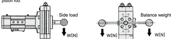
**Allowable Side Load on the Piston End**
