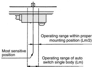
**Operating angle** : The value of the individual auto switch's movement range Lm converted into the shaft's rotation angle
