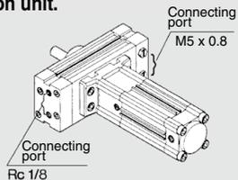
Connecting ports are provided "IN" two positions as standard specifications.
