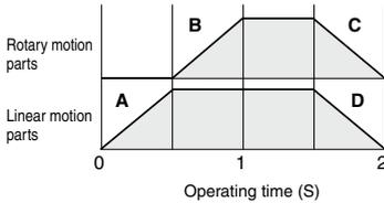
Calculate the amount of air requirement for A, B, C and D respectively.
