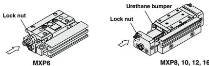
Loosen the lock nut, adjust the stroke with a hexagon wrench from the side marked with an arrow and secure with the lock nut.
