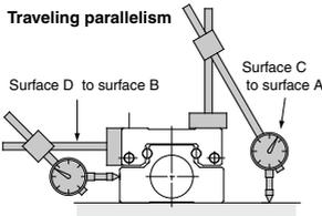
The amount of deflection on a dial gauge when the guide block travels a full stroke with the body secured on a reference base surface.
