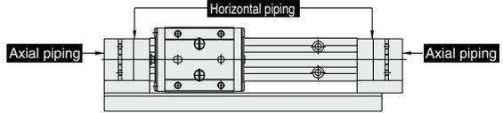
Changing the mounting position of the switch rail, which also used as an air passage can change the direction of the centralized piping.
