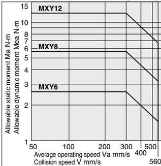
Note) Use the average operating speed when calculating static moment.
