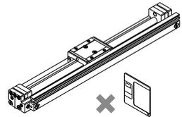
7. Do not attach magnets to the rail and guide block.
