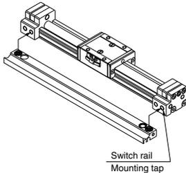
\* Stud fastening: After a temporary tightening, tighten an additional 1/4 turn.
