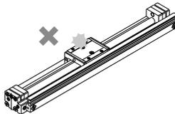
3. Do not apply strong impacts or excessive moment when mounting workpieces.
