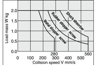
**Table (2) Max. Allowable Load Mass: Wmax (kg)**
