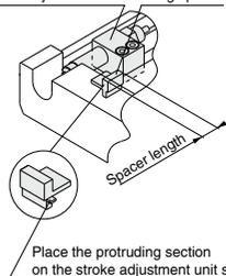
Place the protruding section on the stroke adjustment unit side.
