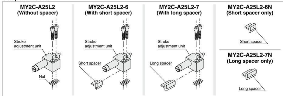
\* Nuts are equipped on the cylinder body.
